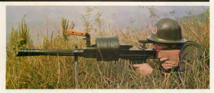
ABOVE: Firing the Type W-87 35mm automatic grenade launcher with 9-round drum from the prone position off its integral bipod. Weight in this configuration is an amazing 26.5 pounds, empty.
